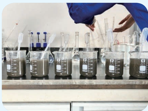
Sludge PAM Flocculant Dosage Experiment
